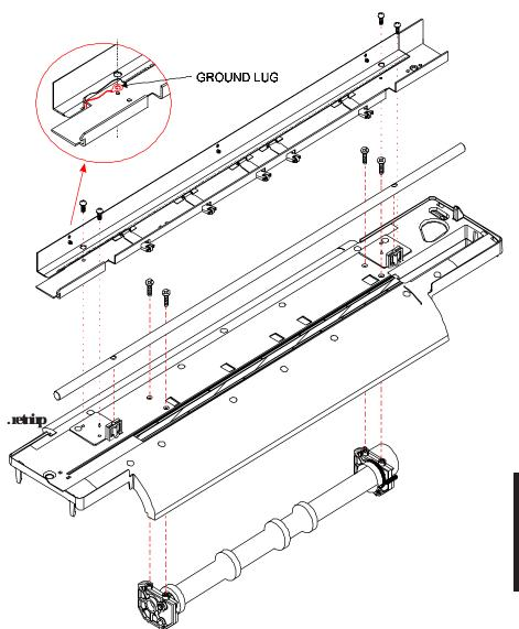
Figure 5-14. C-Bracket Assembly and Platen Removal.
